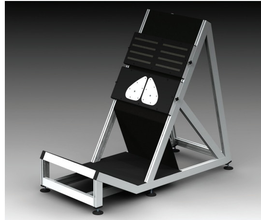
right: CAD Image of the Bodysshelf, showing the position of vibrating actuator plates drawing: Steve Curran, Upside Solutions
